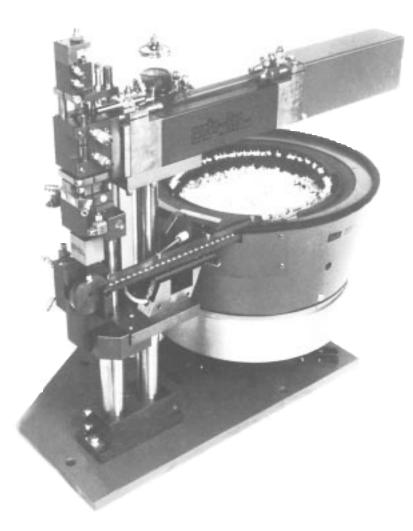
Complete turnkey loading station comprising modular automation elements.
